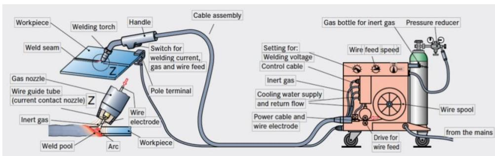
Graphic: Inert gas metal arc welding (TIG/TAG)
