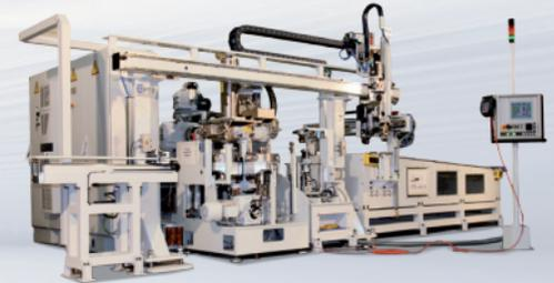
Fully automatic, chained PTR welding lines with loading and unloading as well as upstream and downstream production stages in production lines.
