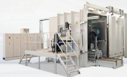
With the EBOMOVE machines with internal mobile generator the welding takes place with linear movements, or by rotating and tilting the EB generator and moving the longitudinal slide.
