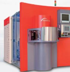
Alternating cycle operation for the manufacture of parts in large volumes. The machines work in this way – exchanging a component at one station while simultaneously welding in vacuum at another.
