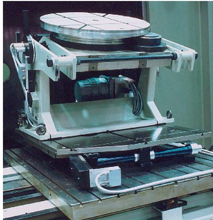
*5-axes workpiece manipulator (47.00.15b)*
