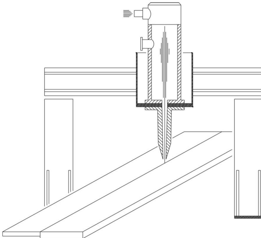
***Electron beam welding
