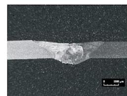
Butt weld, material combination
