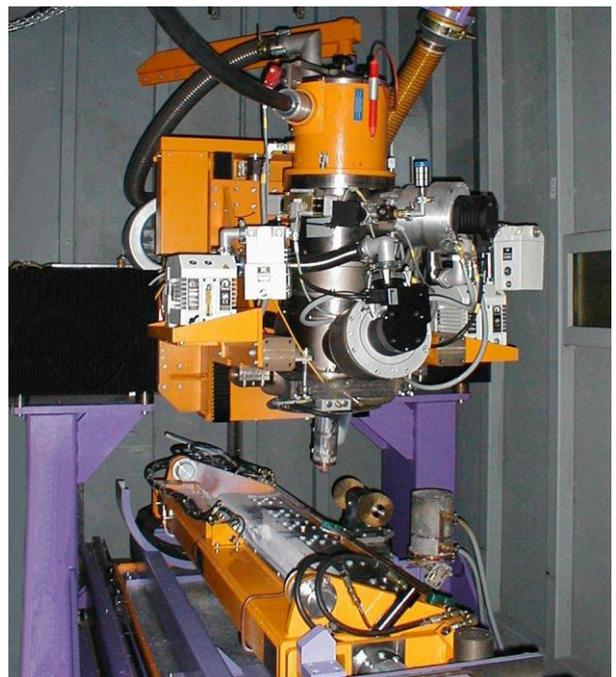
EB generator with portal and clamping device
