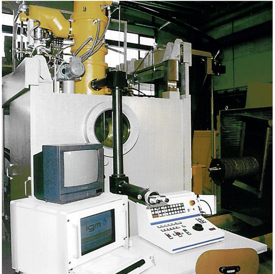
Control console of an EB drilling machine
