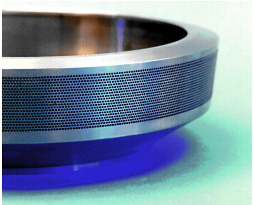
Spinner used in glass fibre production 47.45.01b/7
